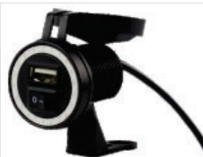
Model: YL-UC16 Material: ABS + Metal Input: 9-24V Output: 5V 2.1A Fit for: Motorcycle/E-Bikes Installation: Handlebar+Rear Mirror Qty/Ctn: 100PCS
