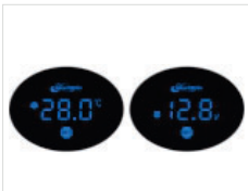
Model: YL-M5542 2-in-1: Voltage, Air temperature Color: Red/Blue/White/Green Fit for: 12V Motorcycle Qty/Ctn: 100PCS
